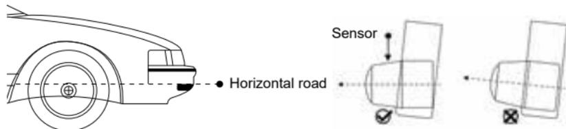
To maintain the optimal detection efficiency, the license plate frame must be kept clear of mud, bugs and other contaminations. There may be situations, when the device signals too late or not at all (f.e.: strong solar radiation, refraction, rainy weather, snow, contaminated sensors). These are not caused by the malfunction of the device, but by the law of physics.
